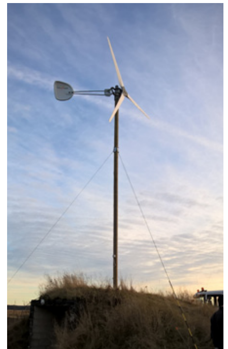
An automatic and reliable storm protection mechanism. The wind generator's storm protection is based on the wind pressure targeted at the rotor.
